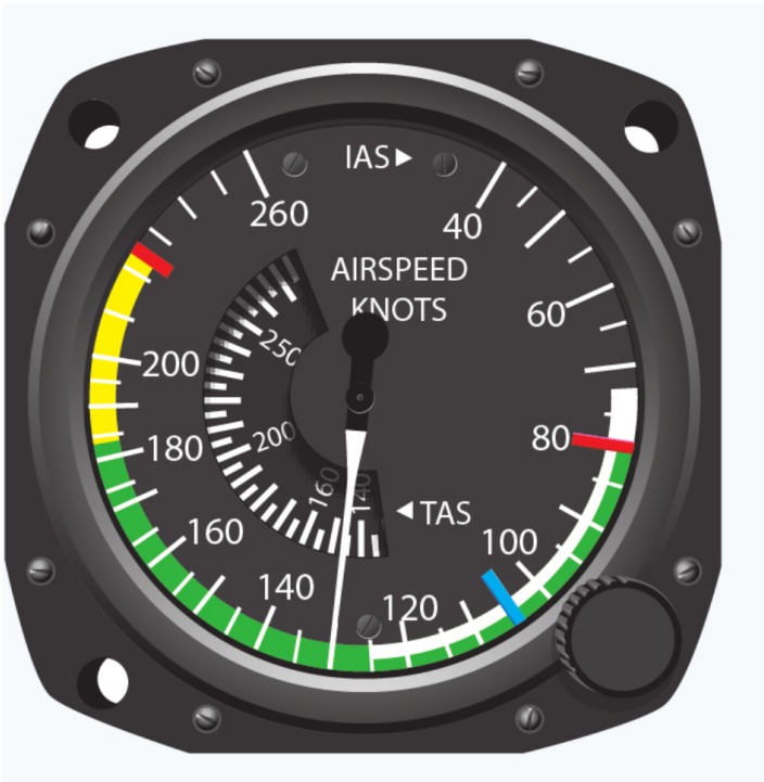
Figure 13-1. Airspeed indicator markings for a multiengine airplane
