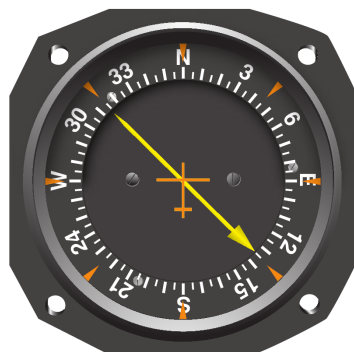
Figure 9-3. Relative bearing (RB) on a fixed-card indicator. Note that the card always indicates 360° or north. In this case, the RB to the station is 135° to the right. If the aircraft were on a magnetic heading of 360°, then the magnetic bearing (MB) would also be 135°.
