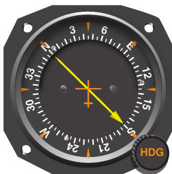
Figure 9-4. Relative bearing (RB) on a movable-card indicator. By placing the aircraft's magnetic heading (MH) of 045° under the top index, the RB of 135° to the right is also the magnetic bearing (no wind conditions), which takes you to the transmitting station.
